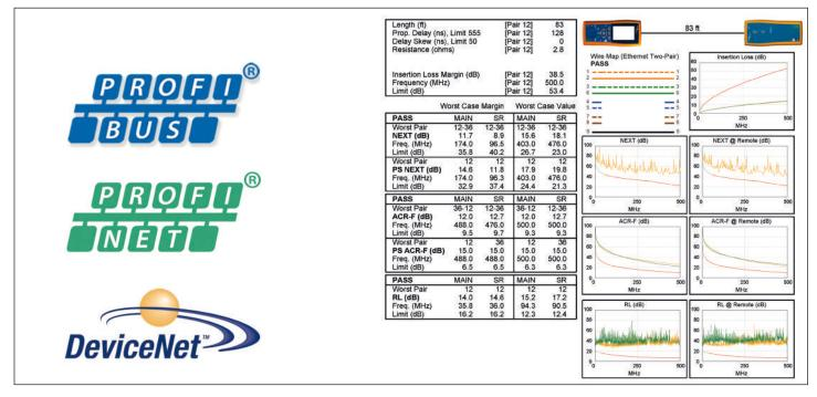
Types of Field Buses of and example of ProfiNET copper cable measurements
