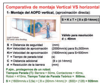
Calculation of vertical ESPE safety distance
