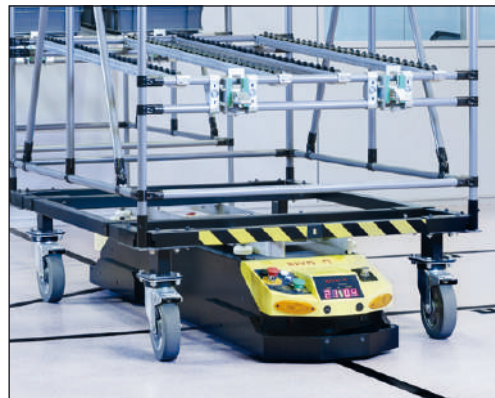
Example of shelving carried by an AGV
